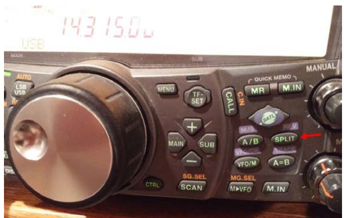
Most modern transceivers have split mode capability with dual VFOs. The red arrow points to the split button on this Kenwood transceiver.
