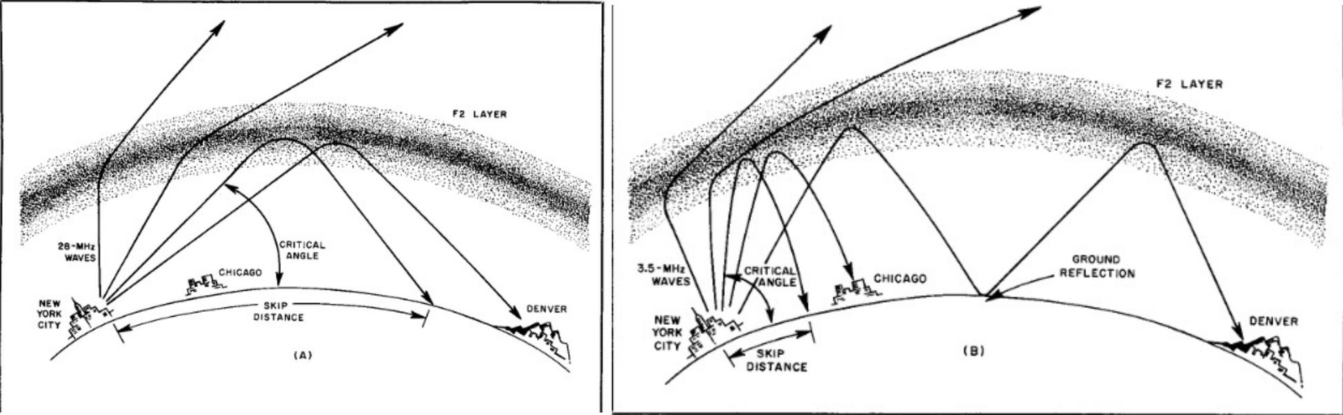
Fig. 6 — Illustration of how frequency, critical angle and skip distance are related. See text for explanation.
