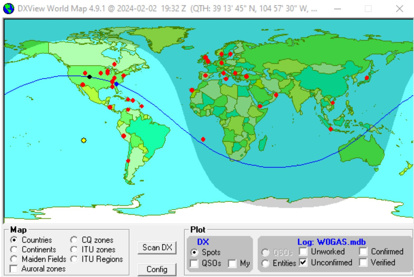
PropView is also part of the DXLabs suite. It auto completes from the panel where I put in the other station's call. Note that it shows current data like SFI (Solar Flux Index) and SSN (Sun Spot Number). Note I can toggle the direction and the path (SP or LP)
