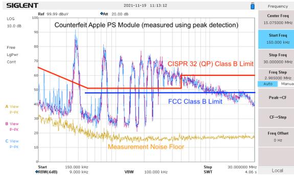
Yellow = ambient noise floor, Violet = Line, Blue = Neutral (Measured from 150 kHz to 30 MHz)
