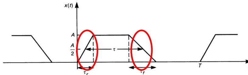
The key contributor to high-frequency harmonic emissions is primarily due to the **rise/fall-times** of the waveform.
