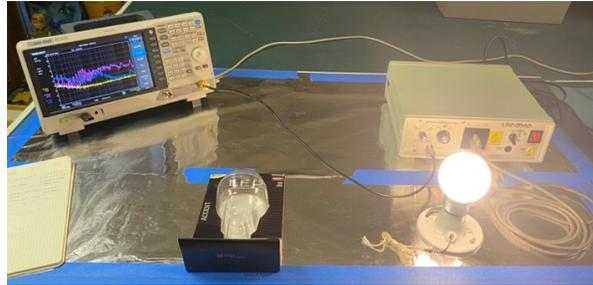
Several LED and CFL bulbs were tested for conducted emissions in the range 150 kHz to 30 MHz at 9 kHz RBW
