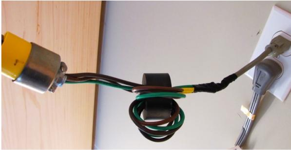
Appliance filter adapter - Bifilar-wound on 2.8 OD #75 core
