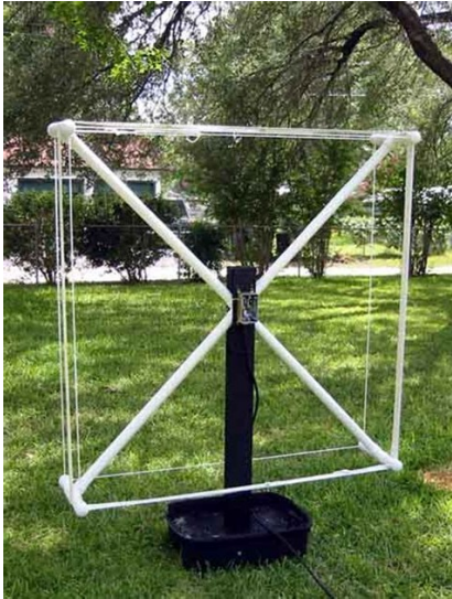
Home-made 1 m wire loop antenna on PVC frame. Can be mounted indoors.
